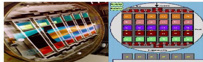
Figure 2 : Actual picture (left) and diagram (right) of arrangement of CCDs. The image of the CCD Camera and the filter transmission plot courtesy of SDSS.
